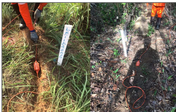
Figure 5: DSU1-508 Accelerometer / Sensor Coupled to the ground from Sismo A team.
